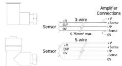
For this reason Positek recommends five wire connections for cable lengths exceeding 10 metres in 0.25 mm<sup>2</sup> cable to preserve the full accuracy of the sensor.
