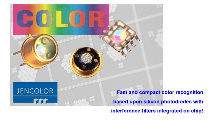
For industrial color applications with high dynamics the new compact color sensors are a preferred choice. Three areas, each of different color, are responsible for the recognition - similar to the human eye. Color sensors based on Si-PIN-diodes and dielectric filters on-chip feature a small design, high-quality filters and the synchronous recording of all three-color ranges.
