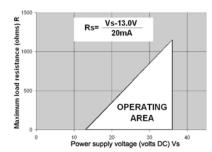
eg with supply voltage load of 36vdc, maximum load is 1150ohms.
